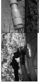
ity to get a leak-tight seal between the polycarbonate straight-through spout and the bushing used to mate the spout to the ½" PVC chamber. Thus this was not a good test of the concept, but more of a problem in translating the concept to a workable, functional prototype. Treatment E (½" lateral lines) appeared to be a very promising candidate in our modeling studies, however the ap-
