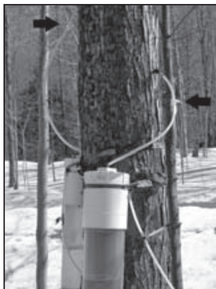
Figure 1. Vacuum chambers for capturing sap from individual tapholes. Arrows point to valves on each dropline that allow the tapholes to be opened or closed.
