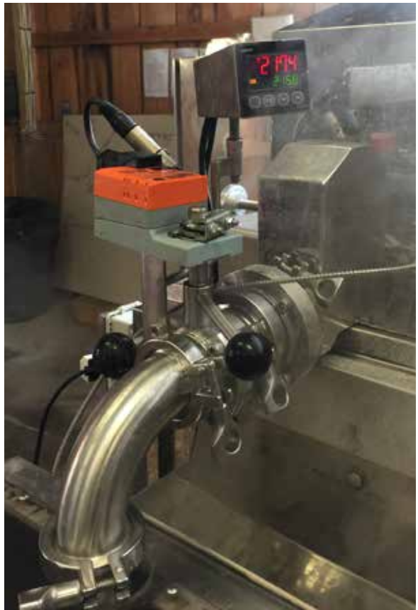
An auto draw-off takes the guesswork out of knowing when syrup is at the right density, and allows for a continuous flow of just-right syrup out of the pan.
