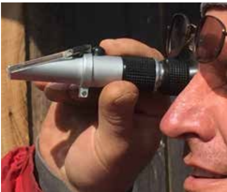
Optical and digital refractometers are excellent tools for testing the density of syrup.
