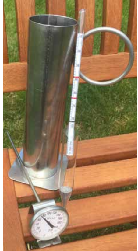
A hydrometer, hydrometer cup, and stem thermometer are inexpensive and important tools for determining syrup density.
