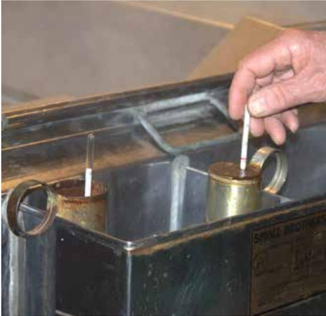
Lower the hydrometer into the cup gently, so it doesn't break. Have at least one spare, in case it does.
