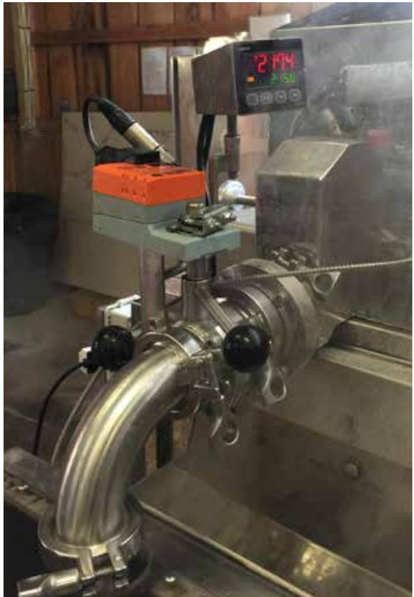
An auto draw-off takes the guesswork out of knowing when syrup is at the right density, and allows for a continuous flow of just-right syrup out of the pan.
