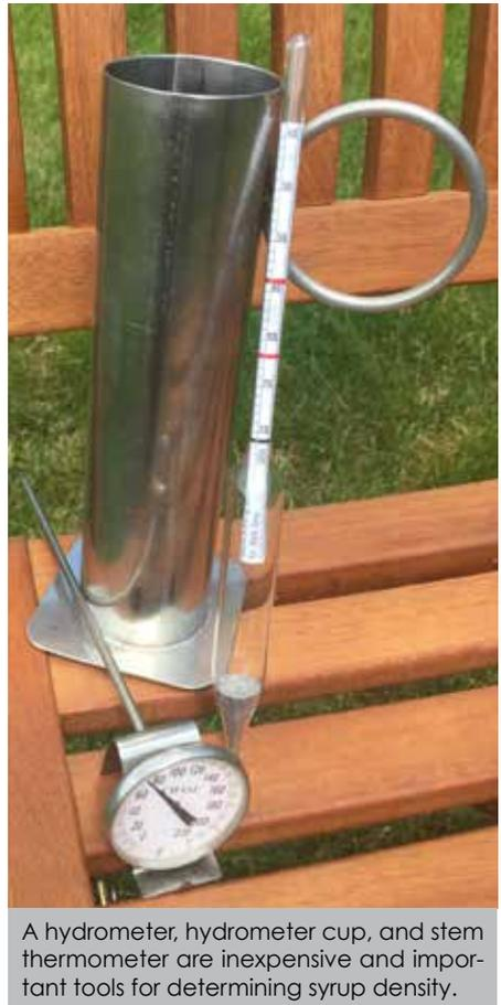
A hydrometer, hydrometer cup, and stem thermometer are inexpensive and important tools for determining syrup density.
