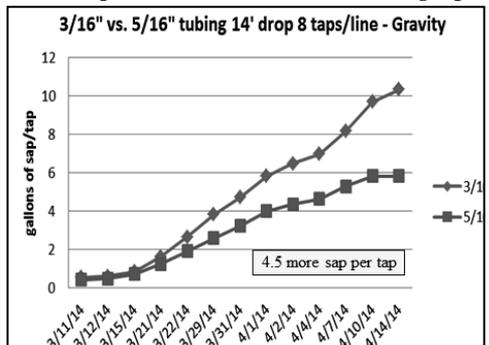
Results from this kind of demonstration create many new questions such as how many taps are needed on a 3/16" line to result in good vacuum and how many taps can a 3/16" line support. This demonstration demonstrates that eight taps seems sufficient to generate significant vacuum, though vacuum tests were not included in this demonstration – it was simply a yield comparison. Testing the number of taps necessary to generate excellent vacuum will need to be conducted during the maple season,
