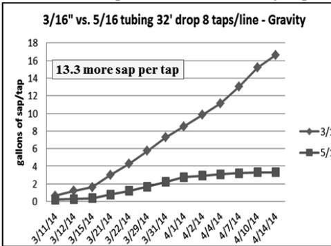
For this experiment, a site was located where we had easy access to the top of the elevation and a drop of 35' was measurable. Water was transported to the site in 15 gallon jugs, and 270' of 3/16" maple tubing was laid on the ground to obtain the drop of 35' on about a 13% slope. The line siphoned water from the jugs to establish the volume of water that could be conducted through the 3/16" lines over time. A
