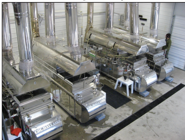
Figure 1. Research evaporators at the University of Vermont Proctor Maple Research Center Maple Processing Research Facility. Evaporators are oil-fueled, 3 × 10' with cross-flow pans and raised flues.
