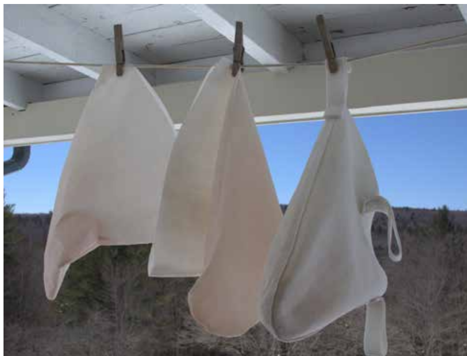
Handle your filters with care, and never wring them out or twist them to dry -- hang them where there is good air circulation. Twisting them will break their fibers, which will allow particles to pass through the next time they are used.
