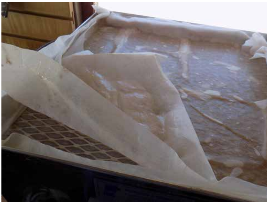
Flat filters are layered over a metal screen which is laid over a pan. The bottom filter is felted wool or synthetic Orlon, and paper pre-filters are laid on top.
