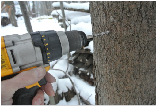
Use a drill bit meant for tapping so that your tap holes are clean and your spiles will seat properly.
