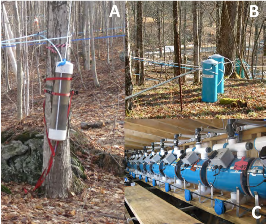
Figure 1. Various methods to measure sap yields from trees under vacuum conditions in sanitation studies. A) Single-tree vacuum chamber, B) Lateral line canisters for multiple trees (typically 3-5), and C) releasers connected to mainlines with 60-120 trees each.
