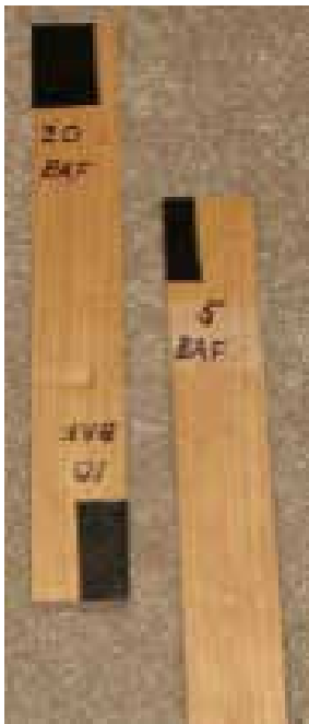
Figure 4: A 'poor man's angle gauge' and determining if a tree is 'in' or 'out.'
