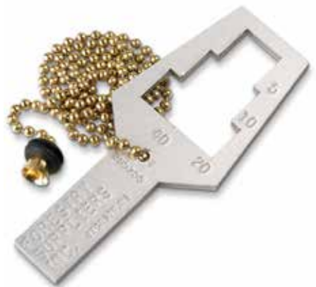
Figure 2: Basal area prism, (left). Basal area angle gauge (right).
