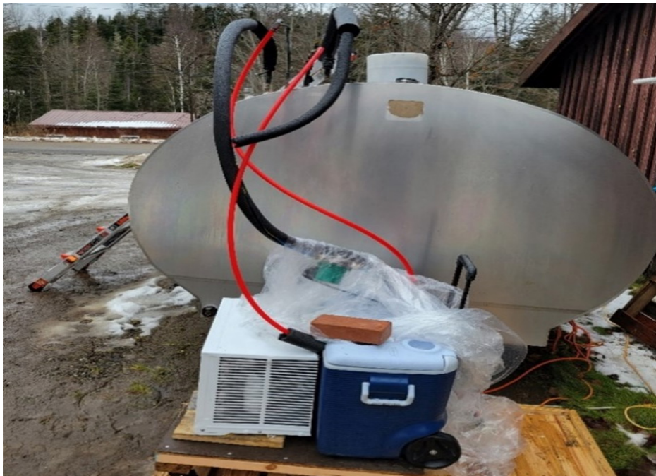
Image 1: DIY glycol chiller connected to a 1,500 gallon tank for testing at the Uihlein Forest
