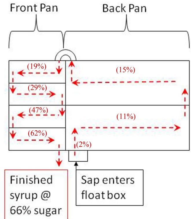
Continuous flow evaporator diagram. Numbers represent % sugar at that location in the evaporator.
