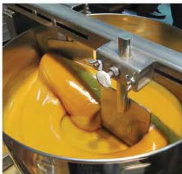
Maple cream is simply maple syrup that has been heated, cooled and stirred. It's a popular item that's easy to make with a device such as this maple cream machine. Photo by Winton Pitcoff.
