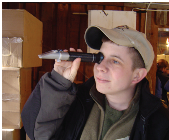
Figure 6. Refractometers are an accurate way to test the concentration of solids (sugars) in the sap to determine when it becomes syrup.
