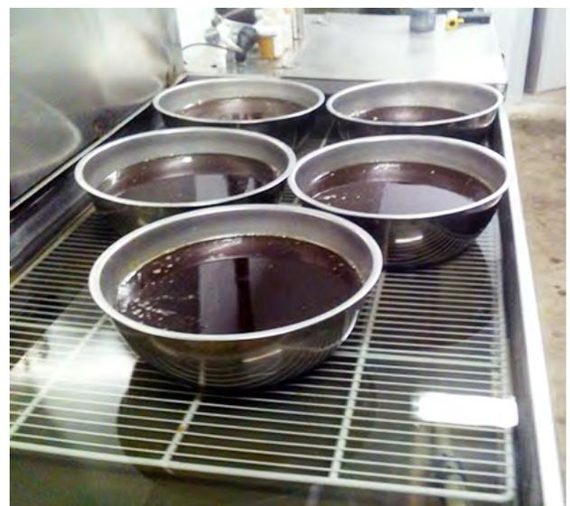
**FIGURE 9.8.** A flowing cold water bath for cooling syrup.
