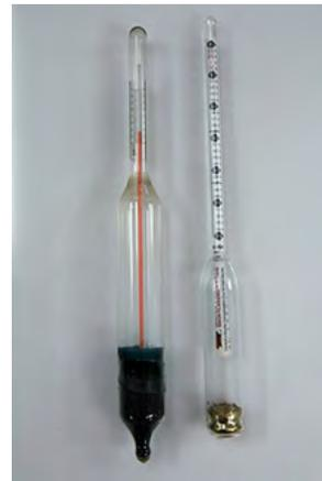
**FIGURE 7.17.** Hydrotherm (left) and hydrometer (right).
