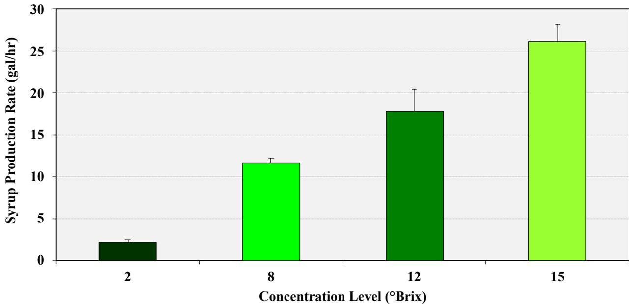
**FIGURE 7.21.** Average syrup production rate (gallons of syrup per hour) in four 3-foot by 10-foot standard evaporators processing sap concentrated to four different levels. ADAPTED FROM: VAN DEN BERG, A.K., T.D. PERKINS, M.L. ISSELHARDT, M.A. GODSHALL, AND S.W. LLOYD. 2011. EFFECTS OF PRODUCING MAPLE SYRUP FROM CONCENTRATED AND RECONSTITUTED SAP OF DIFFERENT SUGAR CONCENTRATIONS. *INT. SUGAR J.* **113**: 35–44.
