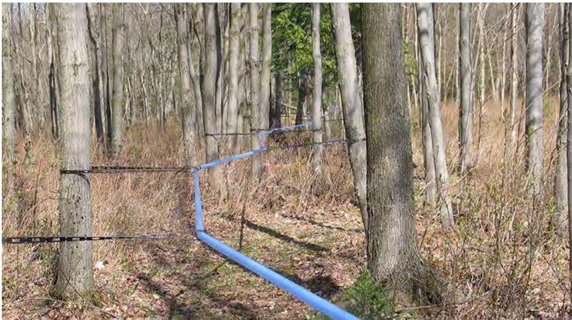
**FIGURE 6.19.** An alternative to standard mainline wire installations, CDL Sugaring Equipment RapiTUBE™ allows quick installation with minimal infrastructure. Proper tensioning is required with this product. Frequent side ties or posts should be used to prevent sagging when the pipe is filled with liquid.
