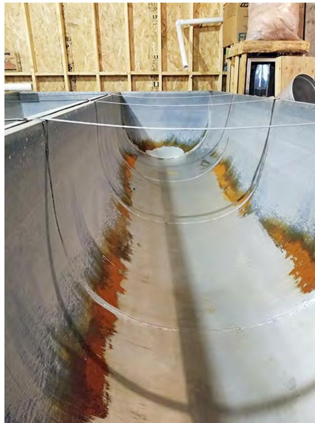
**FIGURE 14.5.** Equipment used for sap collection and storage and for syrup production and storage should be clean, lead-free, and undamaged. This tank is unsuitable and should be retired.
