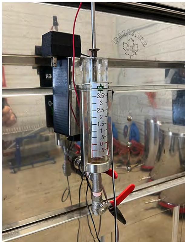
**FIGURE 7.10.** Alarm devices are useful for sounding an alert when liquid level gets low in tanks or pans.
