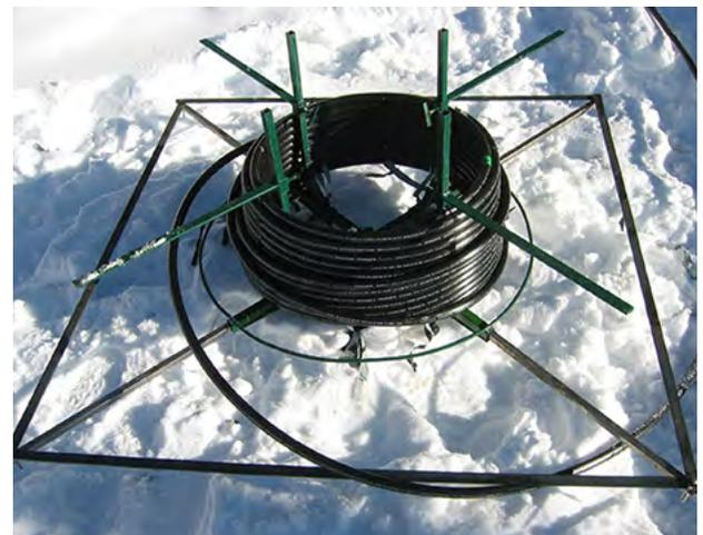
**FIGURE 6.26.** A mainline spooler can be used to easily uncoil tubing as it is pulled into the woods. These are sometimes mounted on ATV-towed trailers for easy transport and maneuvering in the woods.
