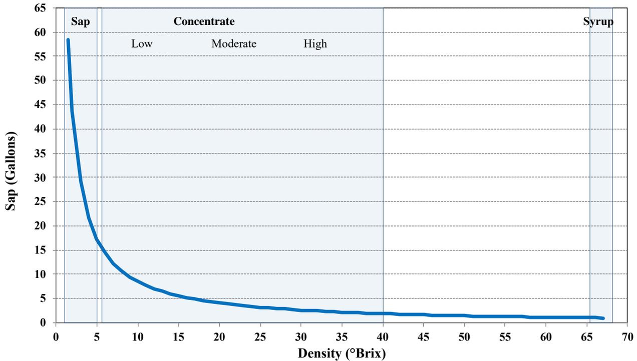
**FIGURE 7.20.** Relationship between the starting sugar concentration of sap and the number of gallons of sap required to produce 1 gallon of maple syrup. The typical Brix ranges of sap, concentrate, and syrup are indicated. ADAPTED FROM: VAN DEN BERG, A.K., T.D. PERKINS, M.L. ISSELHARDT, M.A. GODSHALL, AND S.W. LLOYD. 2011. EFFECTS OF PRODUCING MAPLE SYRUP FROM CONCENTRATED AND RECONSTITUTED SAP OF DIFFERENT SUGAR CONCENTRATIONS. *INT. SUGAR J.* **113**: 35–44.
