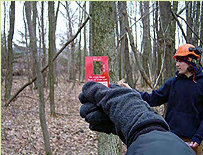
*An angle gauge being used to estimate stand basal area.*
