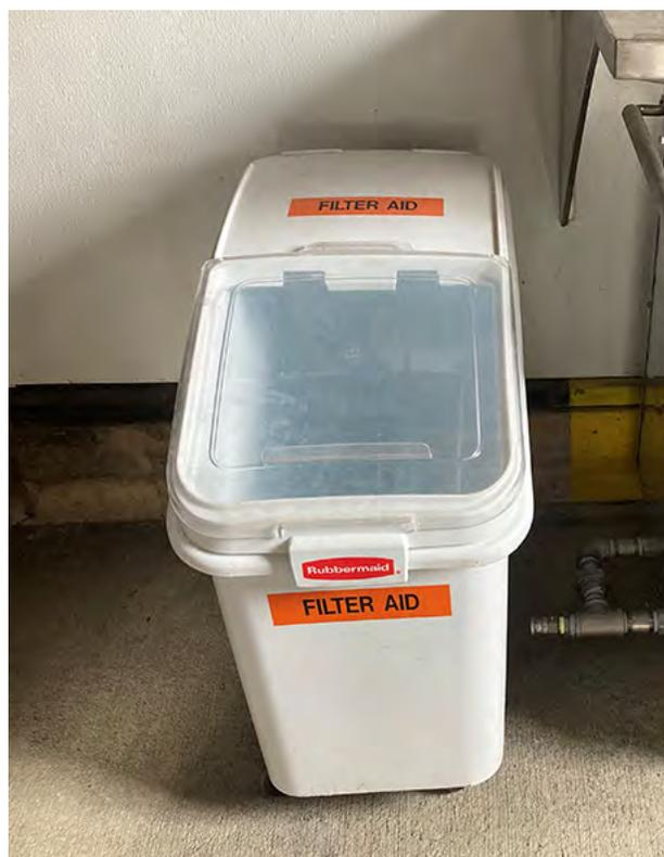
**FIGURE 8.6.** Filter aid should be stored in a food-grade container with a lid so it remains dry and clean for use.
