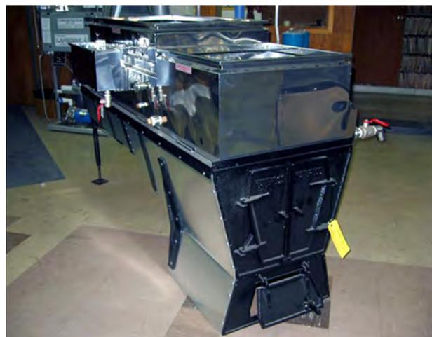
**FIGURE 7.6.** A basic wood evaporator includes vertical sidewalls and a relatively shallow depth to the arch floor beyond the firewall. This maintains the heat close to the bottom of the flues.
