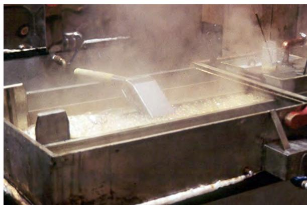
**FIGURE 14.2.** Older lead-soldered and galvanized equipment can leach significant quantities of lead into maple sap and syrup.
