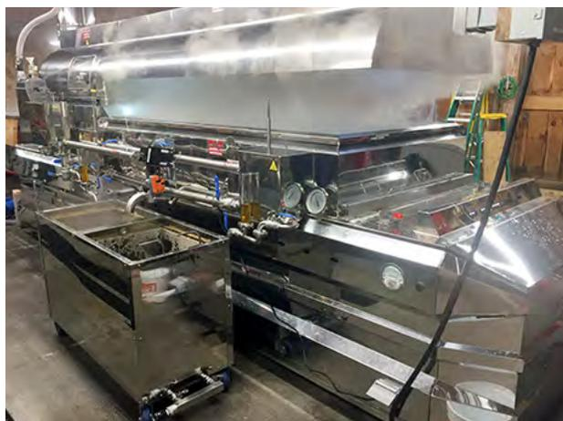
**FIGURE 7.5.** A modern maple evaporator designed for boiling high Brix concentrate, with cross flow pans and a reverse flow option to allow drawing off from one fixed position.
