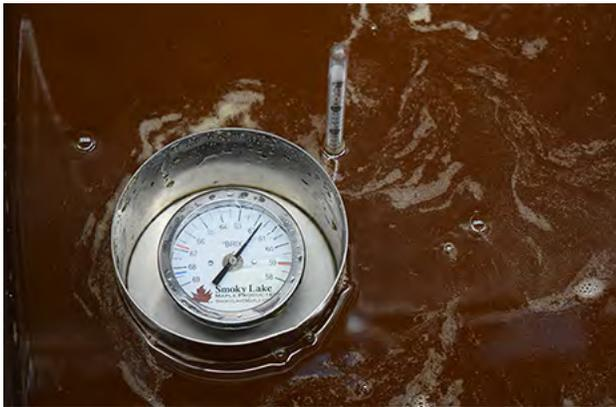
**FIGURE 8.14.** The Smokey Lake Maple Products Murphy Cup™ or Murphy Float™ has a built-in indication of the necessary correction of syrup density. These tools are used in conjunction with a hydrometer. In this example, the hydrometer should read 62.3°Brix for the syrup to be at the correct density.
