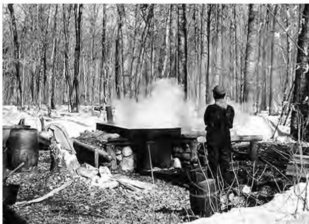
**FIGURE 2.11.** Boiling outdoors on a flat pan setting on a stone arch.
