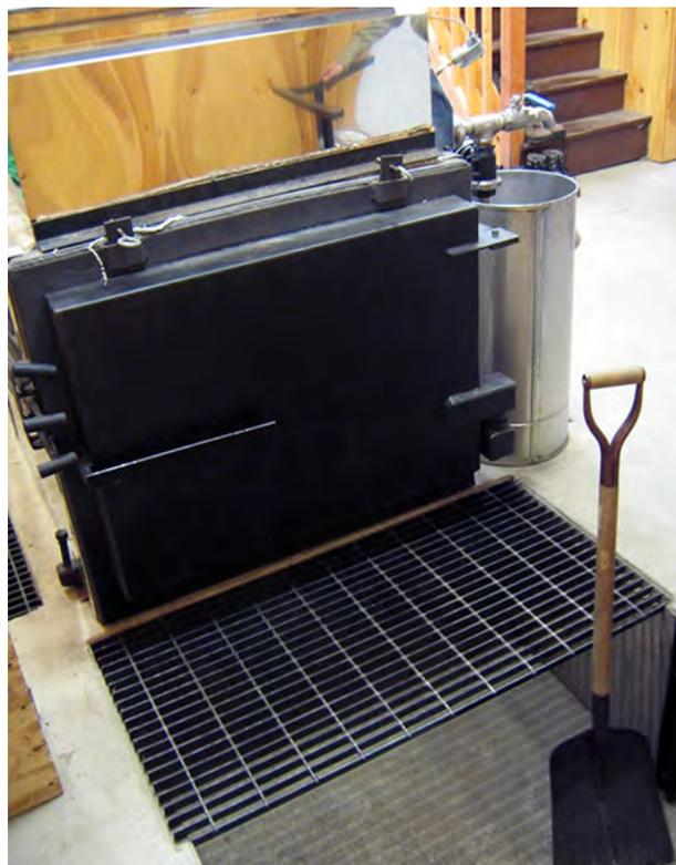
**FIGURE 12.7.** Incorporating a recessed pit in the floor in front of the firebox is a convenient feature in a wood-fired operation.
