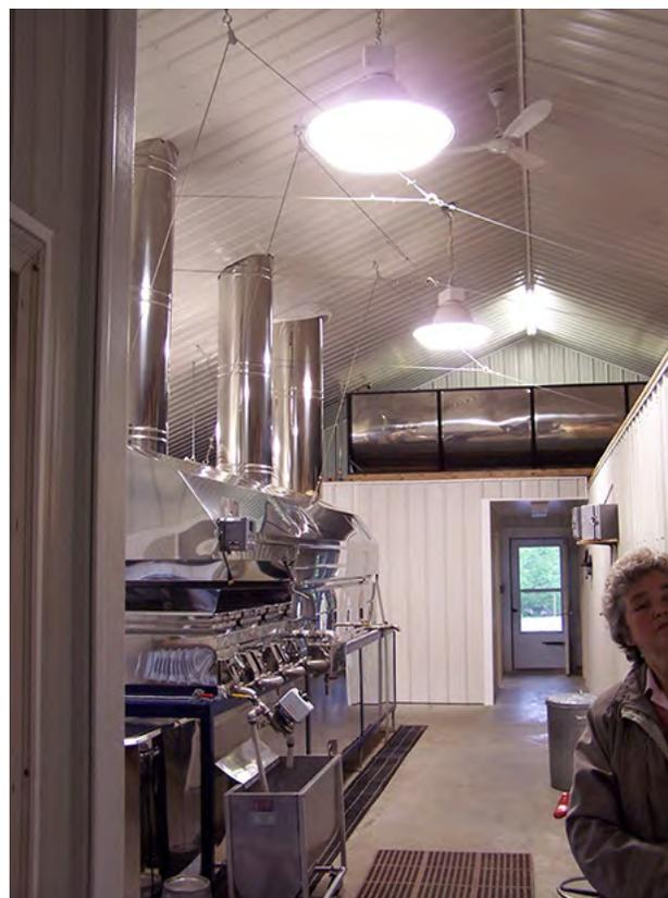
**FIGURE 12.15.** Cables attached to a beam or collar ties can be used to relieve stress on the evaporator from the weight of a “piggyback,” Steam-Away®, or other evaporator accessories.
