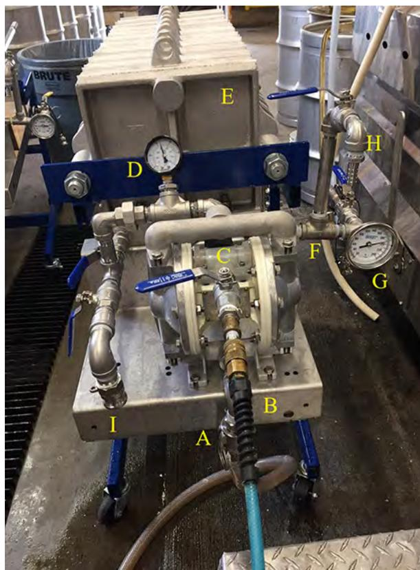
**FIGURE 8.8.** A plate filter press assembled and ready to filter syrup. This press is equipped with an air-powered diaphragm pump. Components include: unfiltered syrup inlet (a), air inlet (b), diaphragm pump (c), pressure gauge (d), plate press and papers (e), filtered syrup outlet (f), temperature gauge (g), filtered syrup sample port (h), and press bypass port (i).
