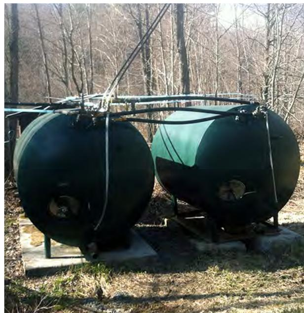
**FIGURE 6.39.** “Zero” tanks in which a vacuum is pulled serve as both extractor and sap storage. These tanks typically have a vacuum rated stamped on them. Exceeding this level can lead to tank collapse.
