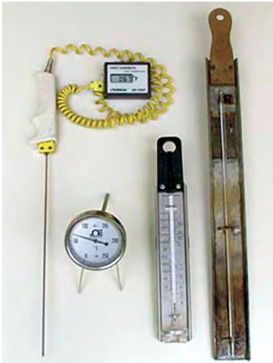
**FIGURE 9.3.** Digital, dial, or stem-type candy thermometers can all be successfully used to make maple confections. Mercury thermometers should never be used in maple syrup or maple product production.
