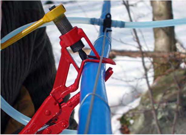
**FIGURE 6.33.** Mainline punch used to drill hole in mainline when installing saddle fitting.
