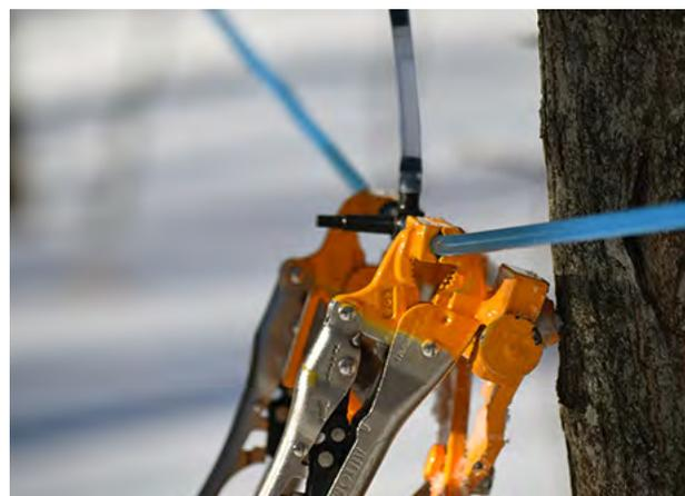
**FIGURE 6.32.** Double-handed tubing being used to install a tee with dropline onto  $\frac{3}{16}$ -inch tubing.
