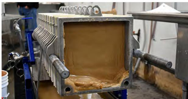
**FIGURE 8.7.** Cake of D.E., sugar sand, and syrup in a filter press after use. Inspection of the cake thickness in relation to the plate cavity will inform the producer of how much filtering capacity has been used in the filtering run.
