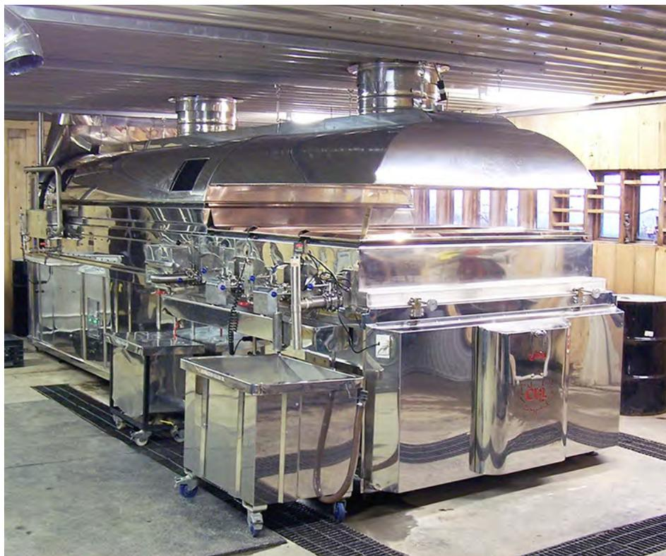
**FIGURE 11.4.** Sap must be processed into syrup quickly via boiling or reverse osmosis in combination with boiling.
