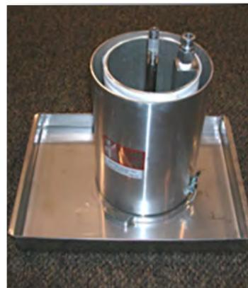
**FIGURE 8.9.** Inner and outer sleeves of a canister pressure filter showing filter cloth wrapped around inner canister. Lid and hoses are not shown.
