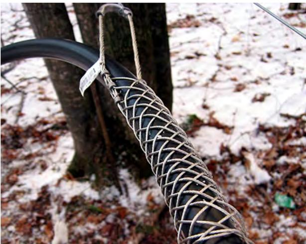
**FIGURE 6.28.** Tubing grip on end of mainline used to pull tubing “hand-tight.”
