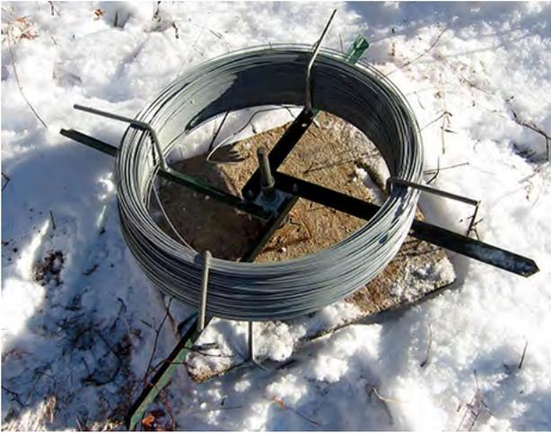
**FIGURE 6.22.** A wire spooler is a useful tool for avoiding kinks when pulling mainline support wire through the sugarbush.
