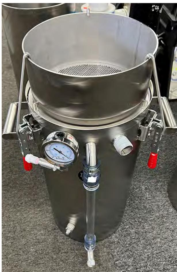
**FIGURE 8.10.** A canister vacuum filter. A filter and pre-filter are placed on the screen in the top section, unfiltered syrup is added, and a vacuum applied to the lower section, drawing syrup through the filter.
