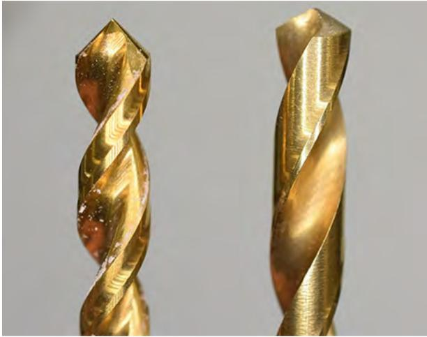
**FIGURE 6.5.** A clean, sharp drill bit designed for tapping maple trees (left) is different from a standard wood bit (right). Tapping bits are made for rapid cutting of fresh wood in live trees and fast removal of wood chips from the taphole. Bits should be replaced if damaged or after about 2,500 tapholes.
