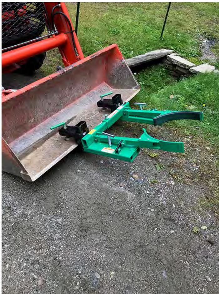
**FIGURE 13.12.** Use mechanical aids such as this barrel lift on a tractor to move heavy loads and prevent back injuries.
