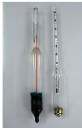
**FIGURE 8.16.** A hydrotherm (on left) and a hydrometer (on right)
