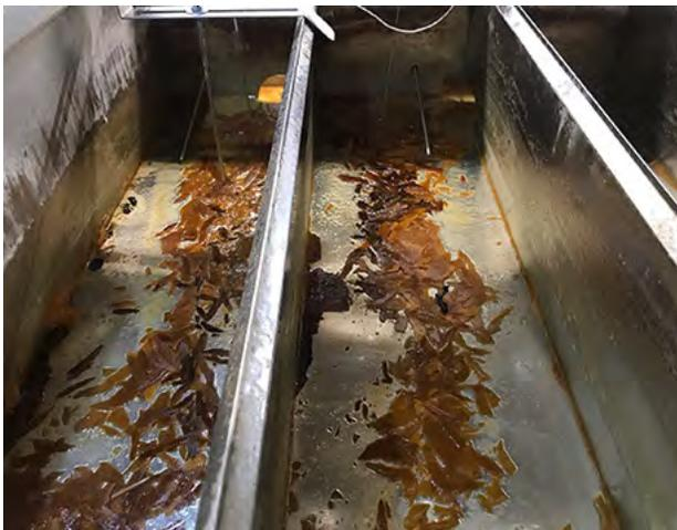
**FIGURE 7.14.** Niter (nitre) in evaporator pans. Niter that is attached is termed “scale” while niter that has flaked off and broken into small pieces and carried along in syrup is called “sugar sand.” Dime for scale.
