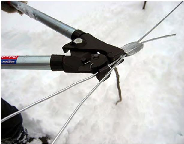
**FIGURE 6.24.** Wire splice (Gripple) being applied to tensioned mainline support wire.
