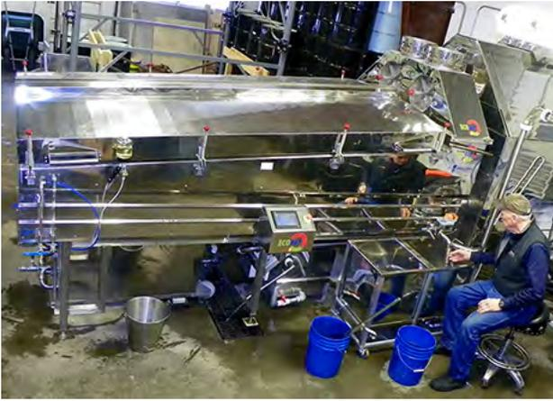
**FIGURE 7.9.** An electric-powered maple evaporator. Note the complete absence of steam, which is condensed within unit and heat energy extracted and recycled.
