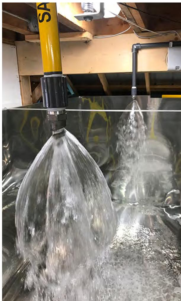
**FIGURE 6.45.** Sap aeration can be useful to retard anaerobic spoilage microorganisms.
