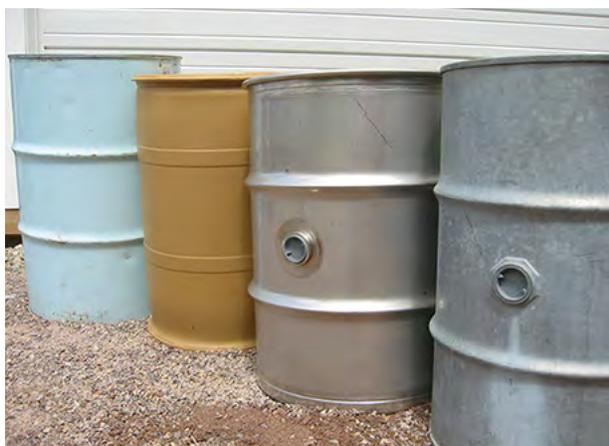
**FIGURE 8.22.** Common types of barrels used in the maple industry include (left to right): epoxy-lined "one-way" steel drums, plastic, stainless, and galvanized barrels. Stainless containers are recommended for maintaining the long-term quality of maple syrup. Galvanized and plastic barrels are being phased out in many locations. Older galvanized barrels with lead solder are no longer appropriate for maple syrup storage.
