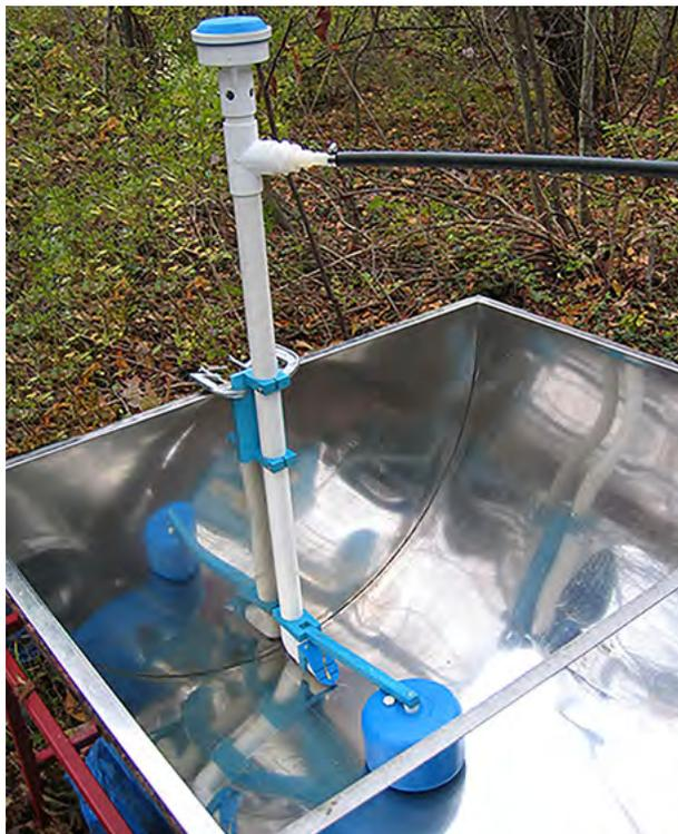
**FIGURE 6.40.** A reverse slope extractor can be used to transfer sap collected from taps situated at an elevation lower than a collection or storage tank.
