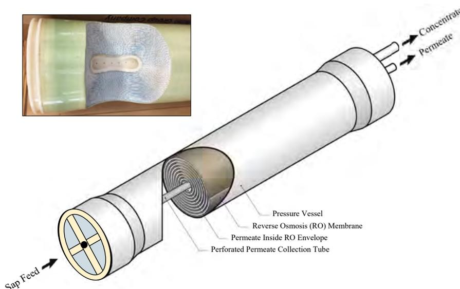
**FIGURE 7.18.** Cutaway diagram of an RO membrane. Sap feeds into the membrane vessel from the lower left. Water passes into the membrane spiral and passes through the membrane before entering the perforated permeate collection tube in the center. Permeate and concentrate exit at the upper right through separate tubes. Inset photo shows an actual maple RO membrane cut to show the inner components.
