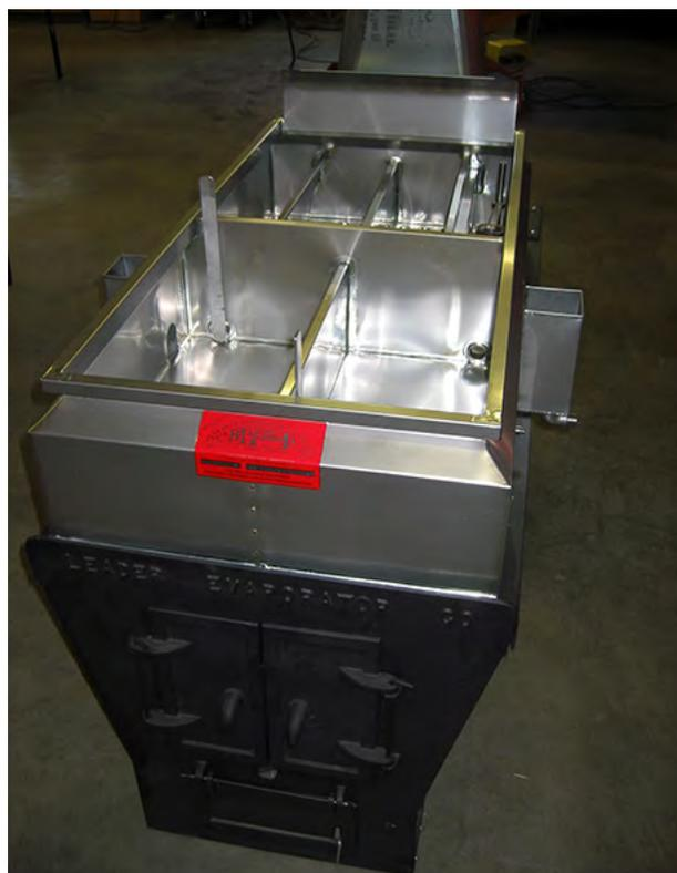
**FIGURE 7.1.** Basic components of a maple evaporator. The arch sits on the floor and contains the heat source (wood in this case). Pans sit upon the top of the arch and hold the boiling liquid. The stack (rearmost in photo) exhausts the excess heat and combustion gases safely out of the vicinity.
