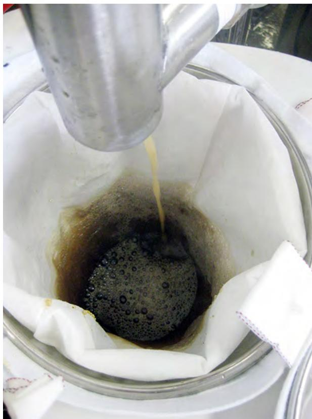
**FIGURE 8.3.** Filtering syrup directly off the evaporator with cone (felt hat) filter and paper prefilter.
