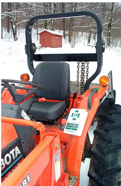
**FIGURE 13.4.** Every tractor and motor vehicle should have a first aid kit. Tractors should always be equipped with a roll-over protective structure.
