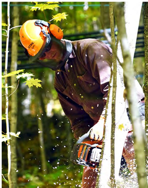
**FIGURE 13.5.** Always wear proper personal protective equipment suitable for the job being performed. Worn or damaged PPE should be promptly retired and replaced.
