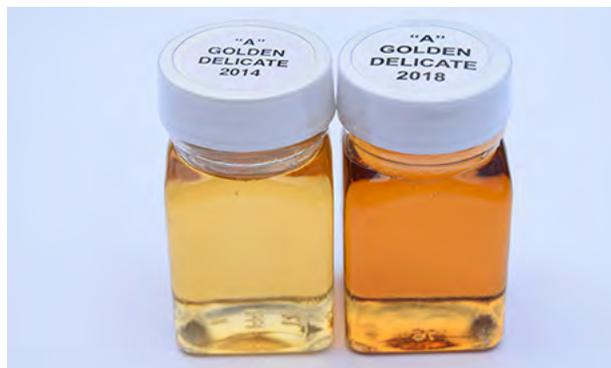
**FIGURE 8.18.** Temporary grading kits will lighten with exposure over time, making any grade determination incorrect.
