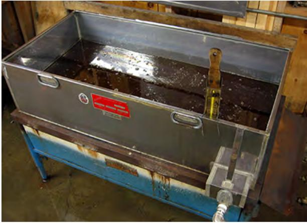
**FIGURE 7.13.** Excessive defoamer use indicated by the oily appearance (rainbow sheen) on top of the syrup in this finishing pan.
