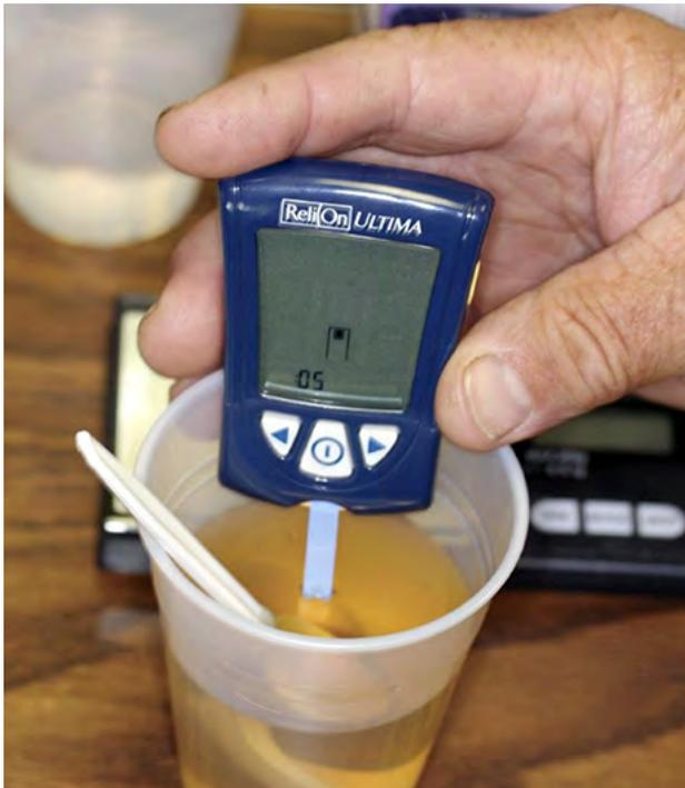
**FIGURE 9.1.** Blood glucose meters can be adapted to test for invert sugar (glucose) in maple syrup.
