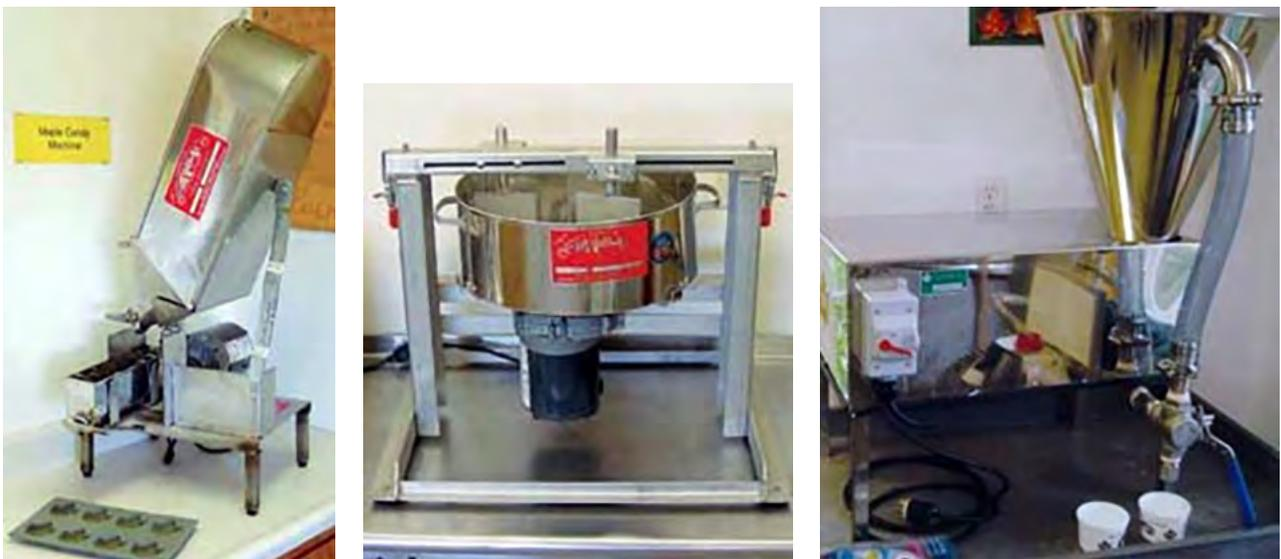
**FIGURE 9.5.** Commercial candy machine (left) and two styles of cream machine (center, right). (DOUGLASS, OBER)
