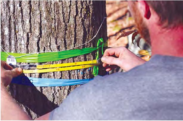
**FIGURE 5.5.** Measuring tree size (dbh) using a diameter tape. If a direct reading diameter tape is not available, measure the circumference and divide by 3.14.
