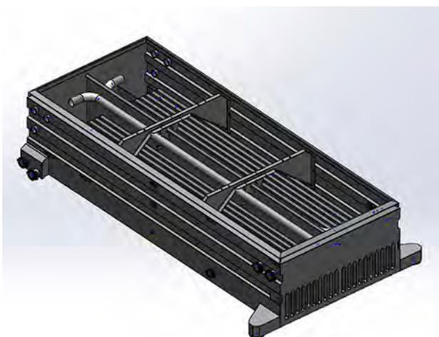
**FIGURE 7.8.** A schematic of a tube-style evaporator flue pan. Hot combustion gases flow through the tubes located near the bottom of the pan from the bottom right to the left. (CDL MAPLE EQUIPMENT)
