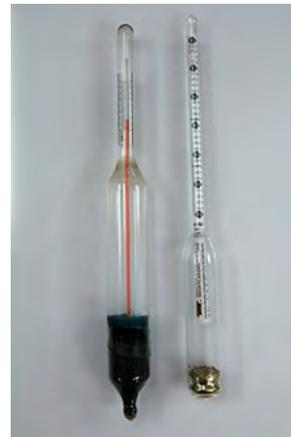
**FIGURE 7.17.** Hydrotherm (left) and hydrometer (right).
