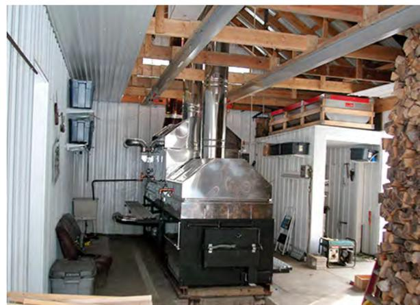
**FIGURE 12.10.** Many sugarmakers add wood storage on to the end of the sugarhouse nearest the arch for easy use.
