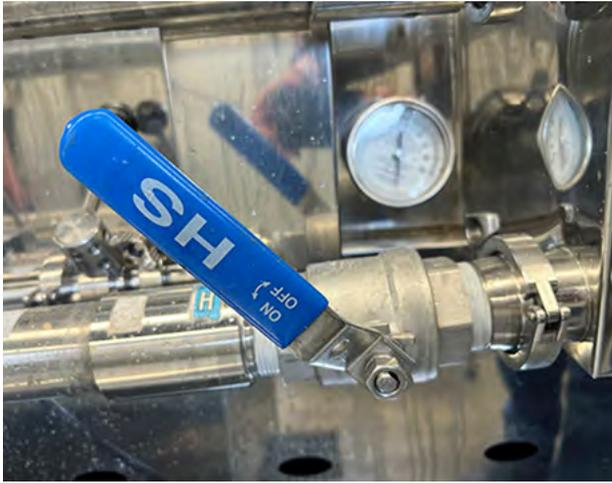
**FIGURE 7.16.** A partially-closed valve positioned between the pan and the draw-off valve can be used to help regulate the flow of syrup at the draw-off and to prevent the liquid level from dropping too low in the syrup pan.
