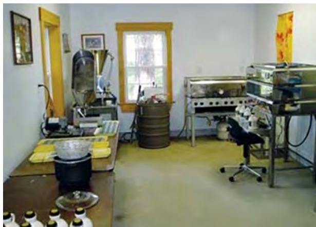
**FIGURE 9.2.** A spacious, clean, ordered, well-equipped area is desirable for making and packaging maple products. Equipment visible includes container and basket for crystal coating candy (left front), soft sugar candy machine with molds (left middle), maple cream machine (left rear), syrup barrel (rear center), propane-fired syrup reheating pan (right rear), canister pressure filter (right middle on floor), and syrup canning equipment (right front). (OBER)
