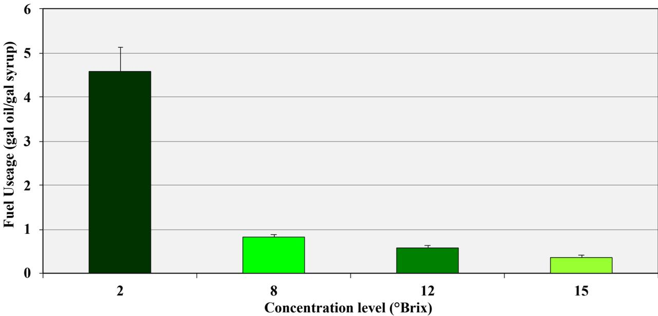
**FIGURE 7.22.** Average amount of oil required to produce a gallon of syrup in four 3-foot by 10-foot standard evaporators processing sap concentrated to four different levels. FROM: VAN DEN BERG, A.K., T.D. PERKINS, M.L. ISSELHARDT, M.A. GODSHALL, AND S.W. LLOYD. 2011. EFFECTS OF PRODUCING MAPLE SYRUP FROM CONCENTRATED AND RECONSTITUTED SAP OF DIFFERENT SUGAR CONCENTRATIONS. *INT. SUGAR J.* **113**: 35–44.
