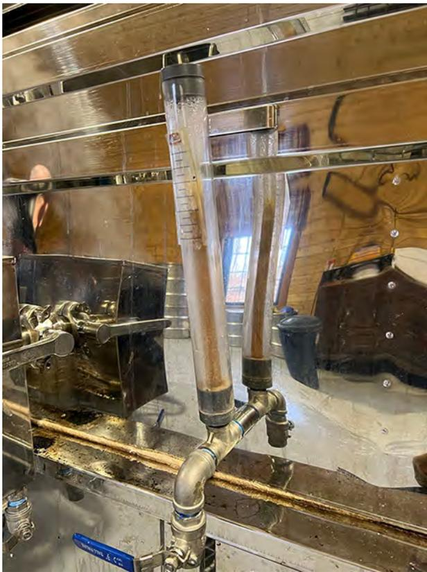
**FIGURE 7.11.** Liquid sight level indicators placed in both the front and back pans allow the operator to tell at a glance if there is a problem with sap/syrup depth.
