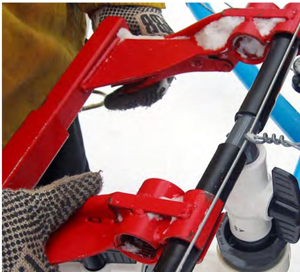
**FIGURE 6.29.** Mainline installation tool, which grips the tubing (top) and holds it in place while it is cut (center), then pushes the tubing over both sides of the fitting by turning a crank that closes the tool (bottom).
