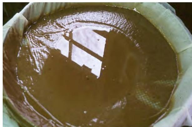
**FIGURE 8.4.** Flat gravity filter/bottling system showing filter sheet and paper prefilter (on top of “felt” filter) and supporting screen.
