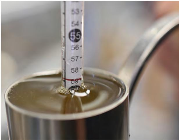
**FIGURE 8.13.** Maple syrup hydrometer floating in a hydrometer cup.
