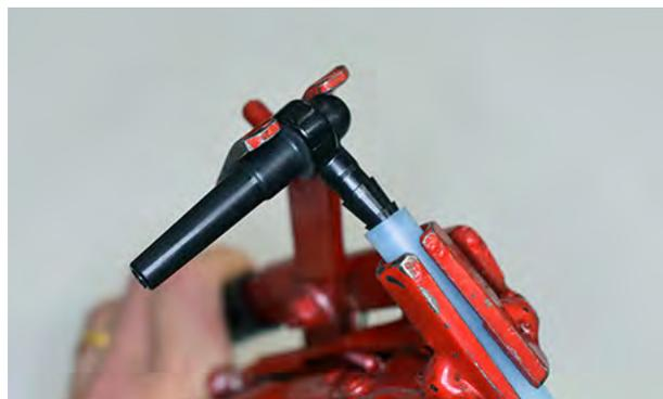
**FIGURE 6.31.** Single-handed tubing tool being used to install a spout onto  $\frac{5}{16}$ -inch tubing.
