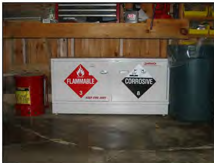
A chemical storage cabinet in a sugarhouse. These cabinets are a great way to store chemicals safely. They minimize the extent of spills, contain small fires and keep chemicals dry, away from incompatible chemicals, food and the public.
