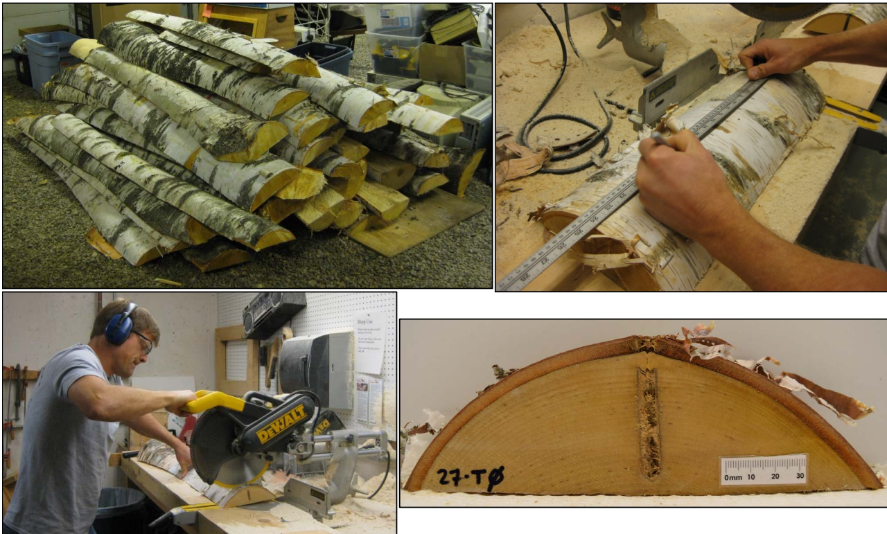
Figure 3. Stem sections from paper birch trees felled for quantification of the volume of nonconductive wood (NCW) associated with taphole wounds. Each segment was cut into 2"-wide cross-sections, photographed, and the area of NCW measured with image analysis software and used to calculate the total volume of NCW associated with the taphole.
