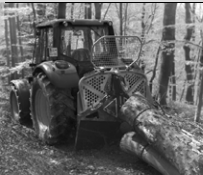
3 pt. hitch Winches Turn your tractor into a skidder.
