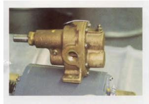
Bronze used in the manufacture of gear pumps usually contains lead, and these pumps can add lead to sap and syrup. Unnecessary pumping, particularly of sap, should be avoided. Other pump models are available which contain little or no lead.
