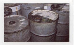
Syrup kept in older, heavy galvanized barrels like these had a much higher lead content after 8 months of storage. Newer galvanized barrels do not add appreciable lead in this amount of time.
