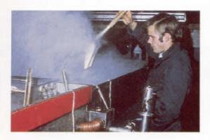
In an **evaporator**, a lead-soldered back pan adds more lead than a lead-soldered front pan, due to the many solder seams. The lead content of partially made syrup often decreases in the front pan, as lead is precipitating and sticking to the pan in the form of sugar sand.
