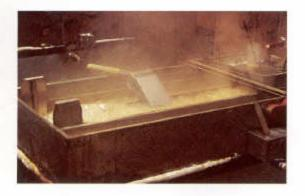
After the evaporator is shut down, lead will continue to accumulate in the partially boiled syrup (sweet) from lead solder. We found that draining the front pan into buckets and adding the sweet again once boiling resumed, reduced lead accumulation.
