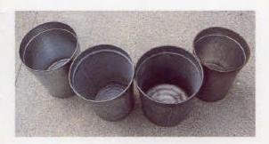
Not all **buckets** are equal when it comes to lead. In our tests, Wheeling buckets (2nd from left) added the least amount of lead, while old "tin" buckets (extreme right) added the most. Some old buckets have shinier terneplate bottoms (3rd from left); beware of these. Lead-free bucket is on the extreme left.
