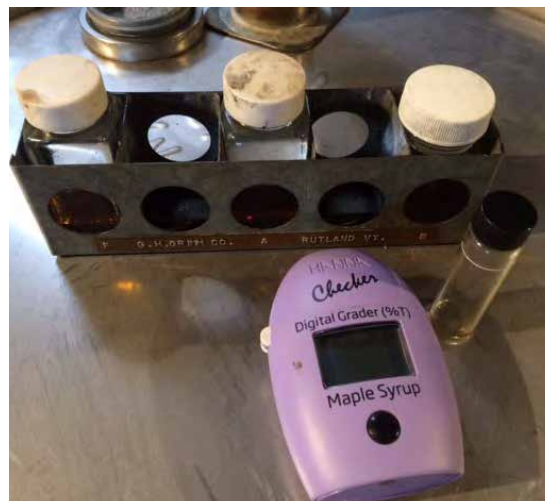
A digital grader for maple syrup. Photo: Cedarvale Maple Syrup Co (NY)
