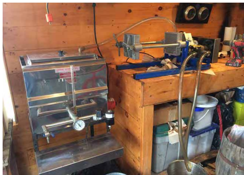
Filter Press and Bottling System. Photo: Josh Penick, Hijinks Farm (NH)
