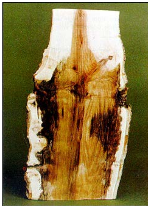
Figure 2. (Left) Bolt showing a closed horizontal scar. (Right) The same bolt sectioned to show internal condition. In this case, the larva was unable to survive to maturity and damage was limited to staining.
