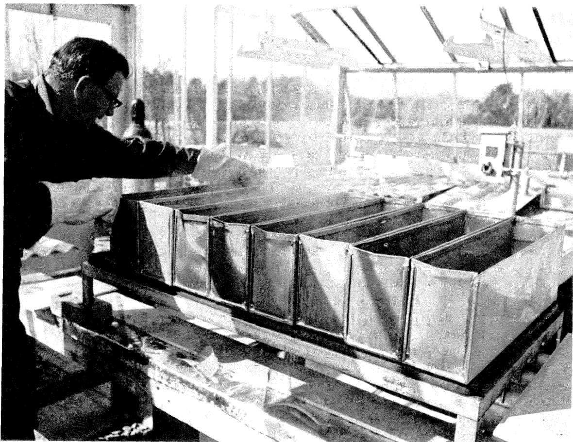
Figure 3.—Each sap sample was concentrated by boiling in a separate open stainless steel pan.
