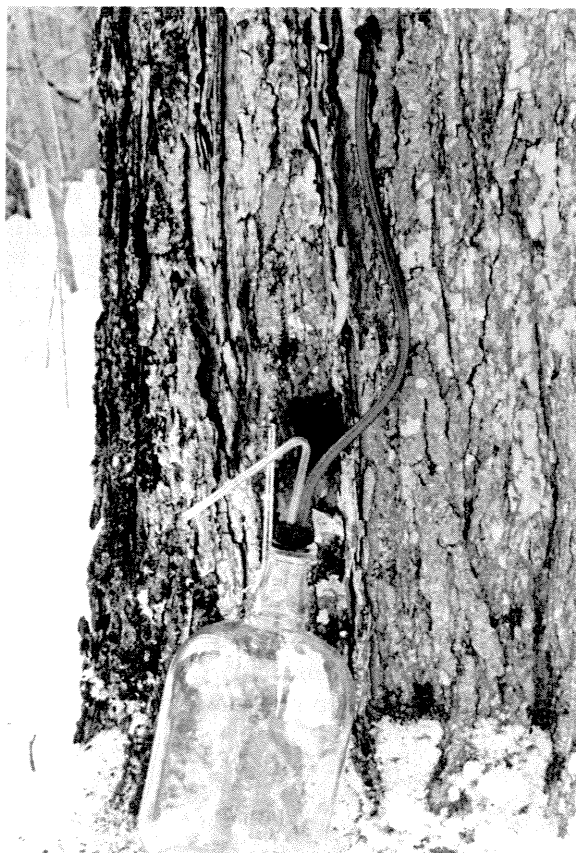
Figure 2.—Glass jug and apparatus for collecting maple sap under sterile conditions.
