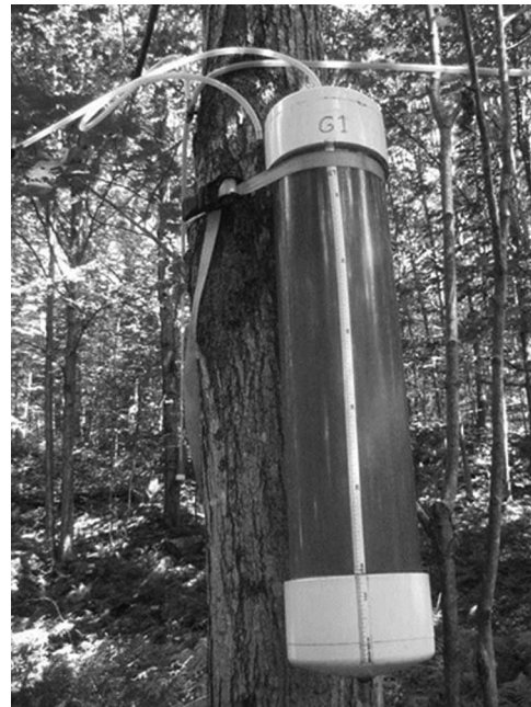
Figure 1. Xylem sap extraction chamber for gravity or vacuum extraction attached to sugar maple ( Acer saccharum ) stem.
