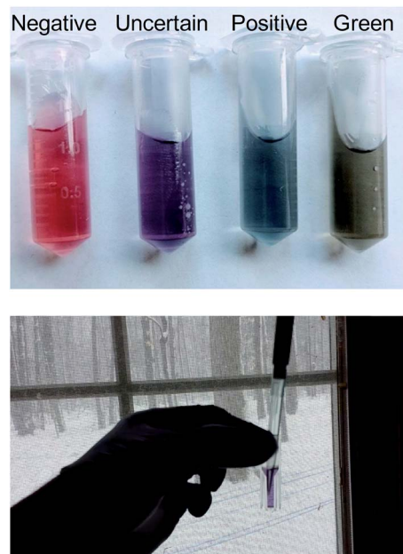
Fig. 6 (Top) Photograph of the different test results (negative: red; uncertain: purple; positive: blue; green: greyish green). (Bottom) Photograph showing a test carried out in a maple sugar shack during the 2018 harvest.
