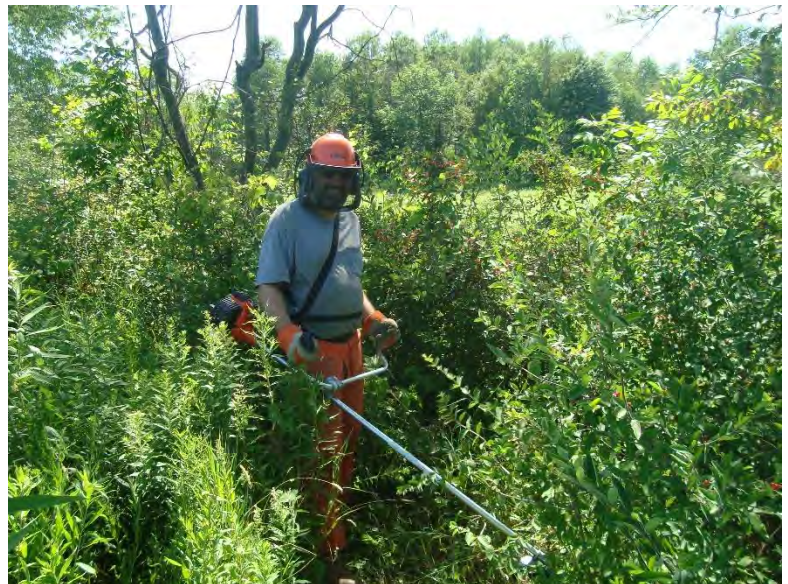
Figure 3. Brush saws can be used as a selective mechanical treatment, or combined with an herbicide to the freshly cut stump to limit sprouting. Personal protective safety equipment is essential.
