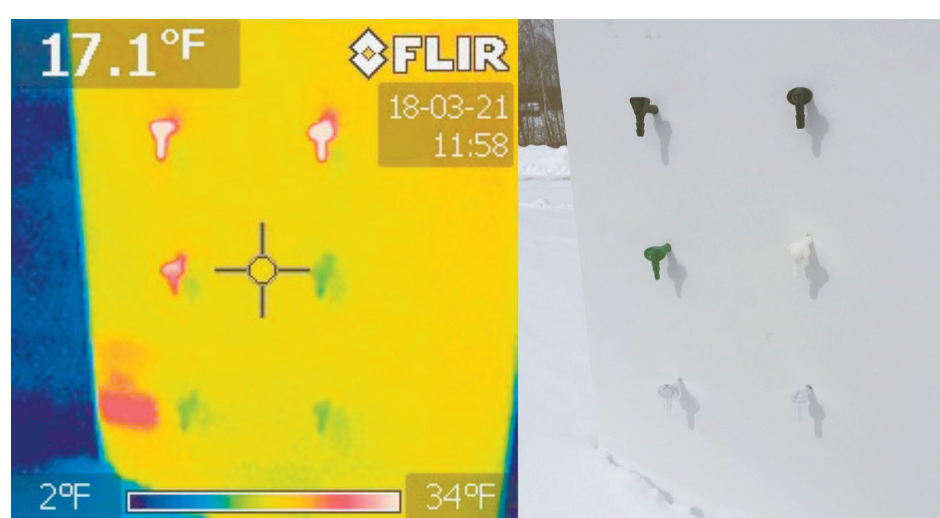
FIGURE 1. Thermal IR (left) and normal color (right) photos of a selection of maple spouts exposed to sun on a cold, wind-less winter day. Ambient temperature is yellow in the IR image. Dark-color spouts show up as warmer (red to white), while white or clear spouts are near ambient temperatures or cooler (yellow to green).
