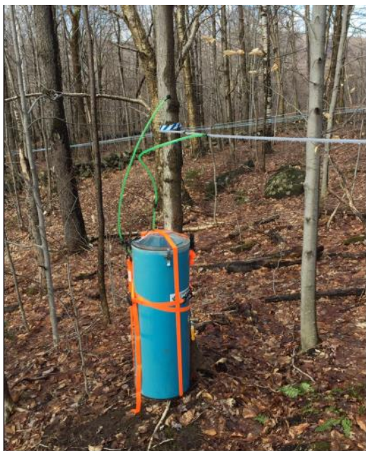
Figure 1. Study tree showing dropline and vacuum chamber for sap collection.
