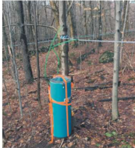
FIGURE 1. Study tree showing dropline and vacuum chamber for sap collection.
