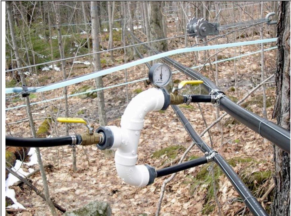
1. A manifold that connects a dry line with a wet line should have a vacuum gauge (Glen Goodrich installation). Shut the valve on the left that leads to the branch mainline. If the vacuum improves, there are leaks along that line that need to be fixed.
