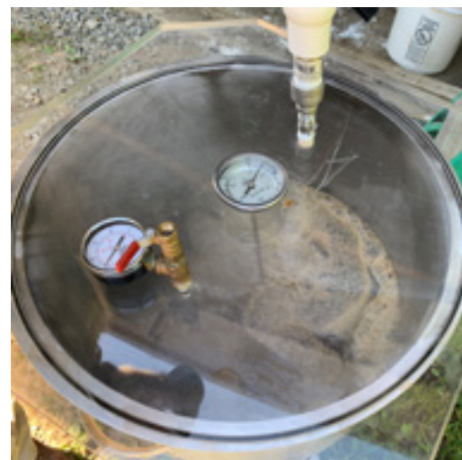
Vacuum boiling vessel
