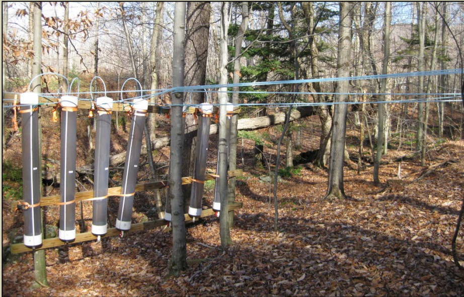
Chambers used to collect and quantify birch sap volume and sugar content under vacuum.
