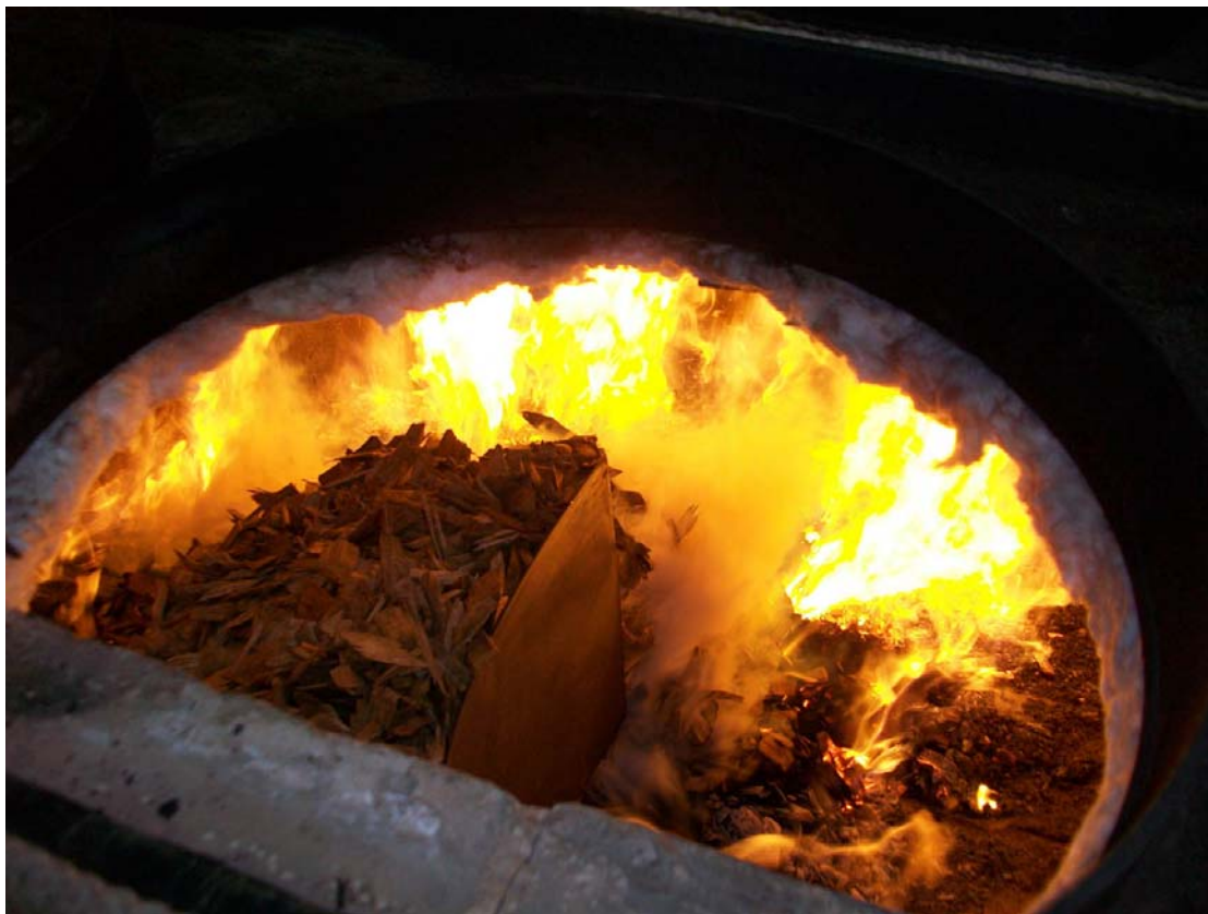
Chips arriving by an auger system in Lee Davis’s evaporator become an inferno in the firebox.
