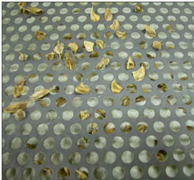
Figure 29 —Chapter 3, Seed Harvesting and Conditioning: the seeds caught in the screen holes are said to have “blinded” the screen.
