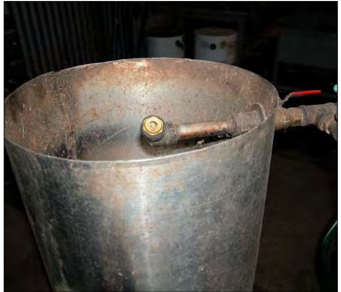
Figure 15 —Chapter 3, Seed Harvesting and Conditioning: a water Chapter 3, valve installed on the side of the macerator improves ease of operation.
