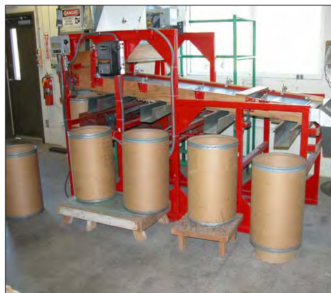
Figure 25 —Chapter 3, Seed Harvesting and Conditioning: cleaner-sizer machine has 5 screens to give 6 separations at once.
