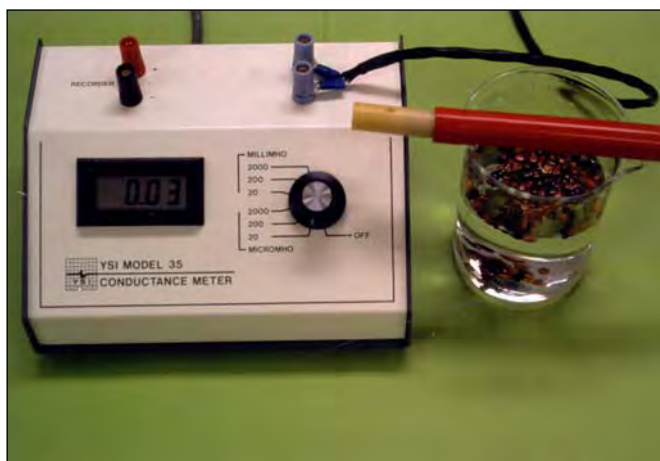
Figure 25 —Chapter 5, Seed Testing: the conductivity meter is used to measure seed viability or vigor by estimating the amount of cations lost from deteriorating seeds.
