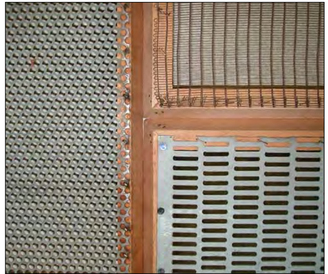
Figure 28 —Chapter 3, Seed Harvesting and Conditioning: hand screens showing the 3 main types of screens used to clean seedlots (counter-clockwise from left): perforated metal round hole, perforated metal oblong holes, and woven wire.
