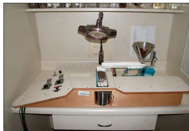
Figure 14 —Chapter 5, Seed Testing: a mechanical purity board can reduce the time required to conduct a purity analysis.
