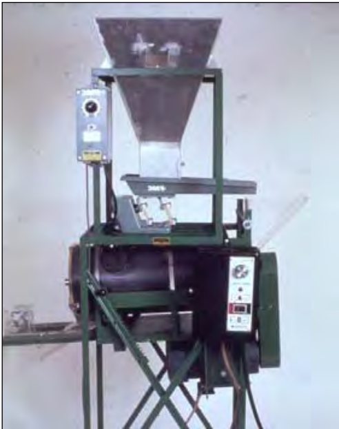
Figure 21 —Chapter 3, Seed Harvesting and Conditioning: small-lot pine-seed de-winger developed by the USDA Forest Service's Missoula Technology and Development Center, Missoula, Montana.
