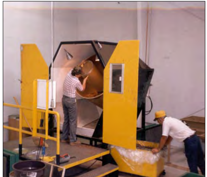
Figure 23 —Chapter 3, Seed Harvesting and Conditioning: commercially made wet pine-seed de-winger.
