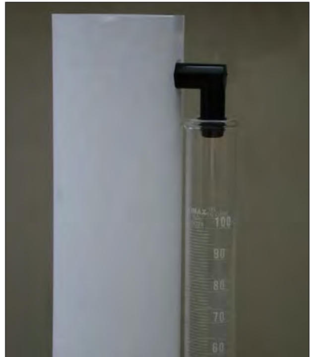
Figure 4 —Chapter 3, Seed Harvesting and Conditioning: two-cylinder system for measuring specific gravity of pine cones.
