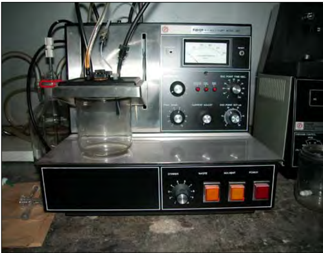
Figure 11 —Chapter 5, Seed Testing: the Karl Fisher apparatus is used as the analytical standard for determining seed moisture content.
