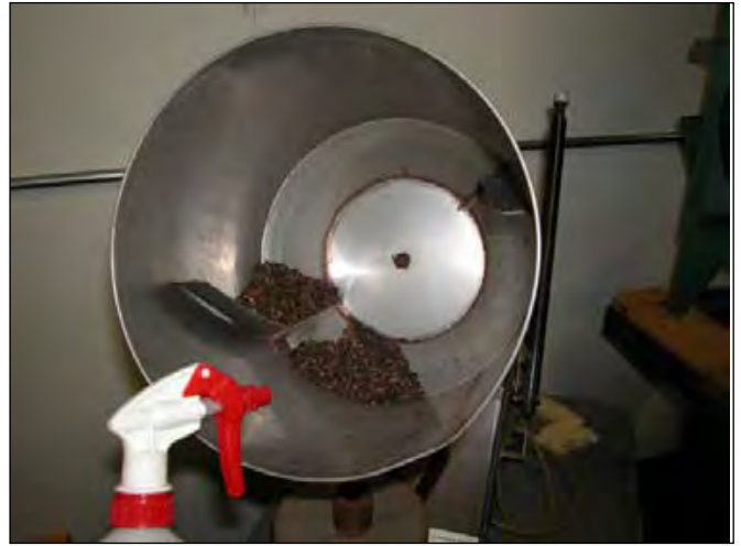
Figure 22 —Chapter 3, Seed Harvesting and Conditioning: small mixer for tumbling seeds for wet and dry de-winging; the spray bottle is used to apply water for wet de-winging.
