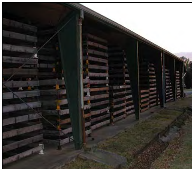
Figure 12 —Chapter 3, Seed Harvesting and Conditioning: screen bottom trays under shelter for air-drying dry fruits.
