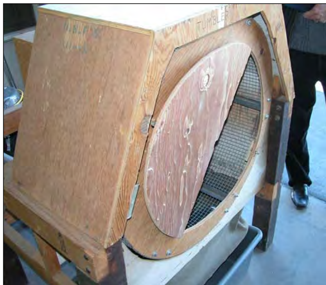
Figure 18 —Chapter 3, Seed Harvesting and Conditioning: a tumbler can be used to extract seed from dehiscent cones or fruits.
